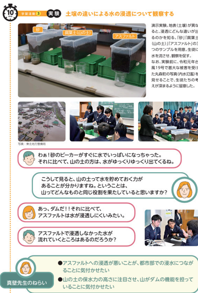
Fig. 1. From the disaster risk reduction Education Booklet. (Left) Students tested how water moves through sand, mountain soil, and asphalt. They observed that mountain soil held water slowly, similar to a dam. The asphalt did not absorb water, causing it to run off. The teacher asked, “Where does the water go in the city?” Students learned how land types affected the floods. (Right) Effective use of web-GIS hazard mapping is explained. GIS, Geographic Information Systems. Adapted from Miyagi University of Education [19] with permission of the copyright holder.
